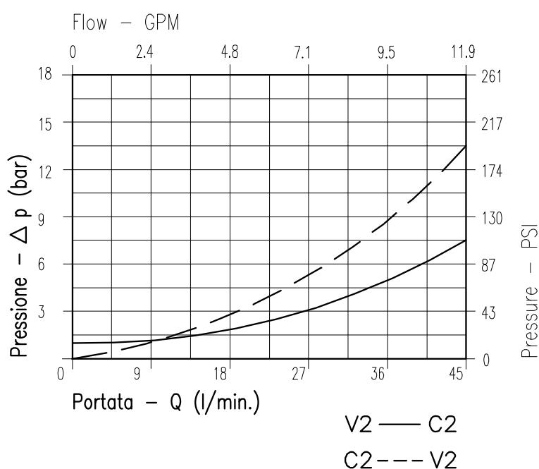
**Viscosità olio 46 cSt a 50°C - Oil viscosity 46 cSt at 50°C**
