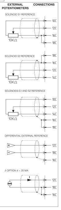
The two available regulations P3 and P4 permit to respectively regulate the ramp times for positive and negative variations of the reference signal. In case of application of the driver in closed loop systems, it is advisable to disable the ramp function: it is possible to permanently disable this function by means of a switch on the card side ( $\boxed{2}$ ) or temporarily, connecting the pin 6c and 6a ( $\boxed{2}$ )
