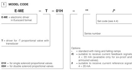
E-ME-T drivers control the current to the solenoid of Atos proportional valves with position transducer, regulating the spool position or the flow according to the electronic reference signal, adjusted by transducer's feedback.
